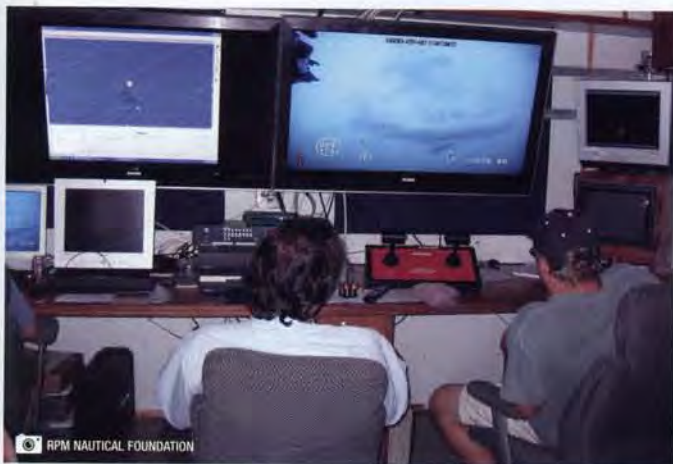
Figure 6: Data from the multibeam positioning model (left) along with video (centre) and sonar (far right) feeds from the ROV are coordinated in the operations room.
