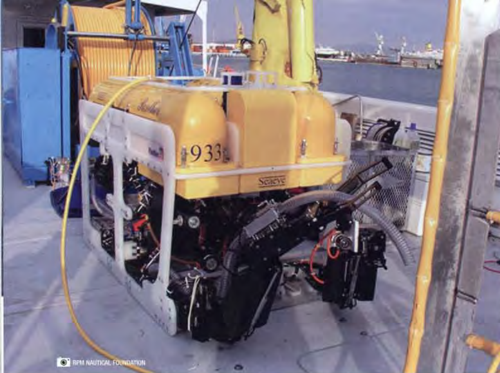
Figure 4: RPM Nautical Foundation's Seave Panther XT ROV used for site discovery, recording, and excavation.
