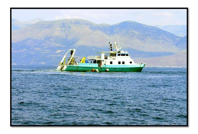
**Length**: 37.3 m / 122 ft **Beam**: 6.7 m / 22 ft **Configuration**: Monohull
